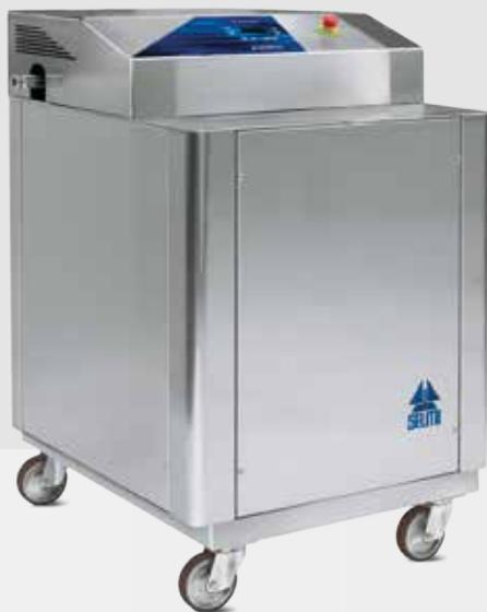
Equipped with a pedal or button controlled screw pump for the extraction of chocolate
